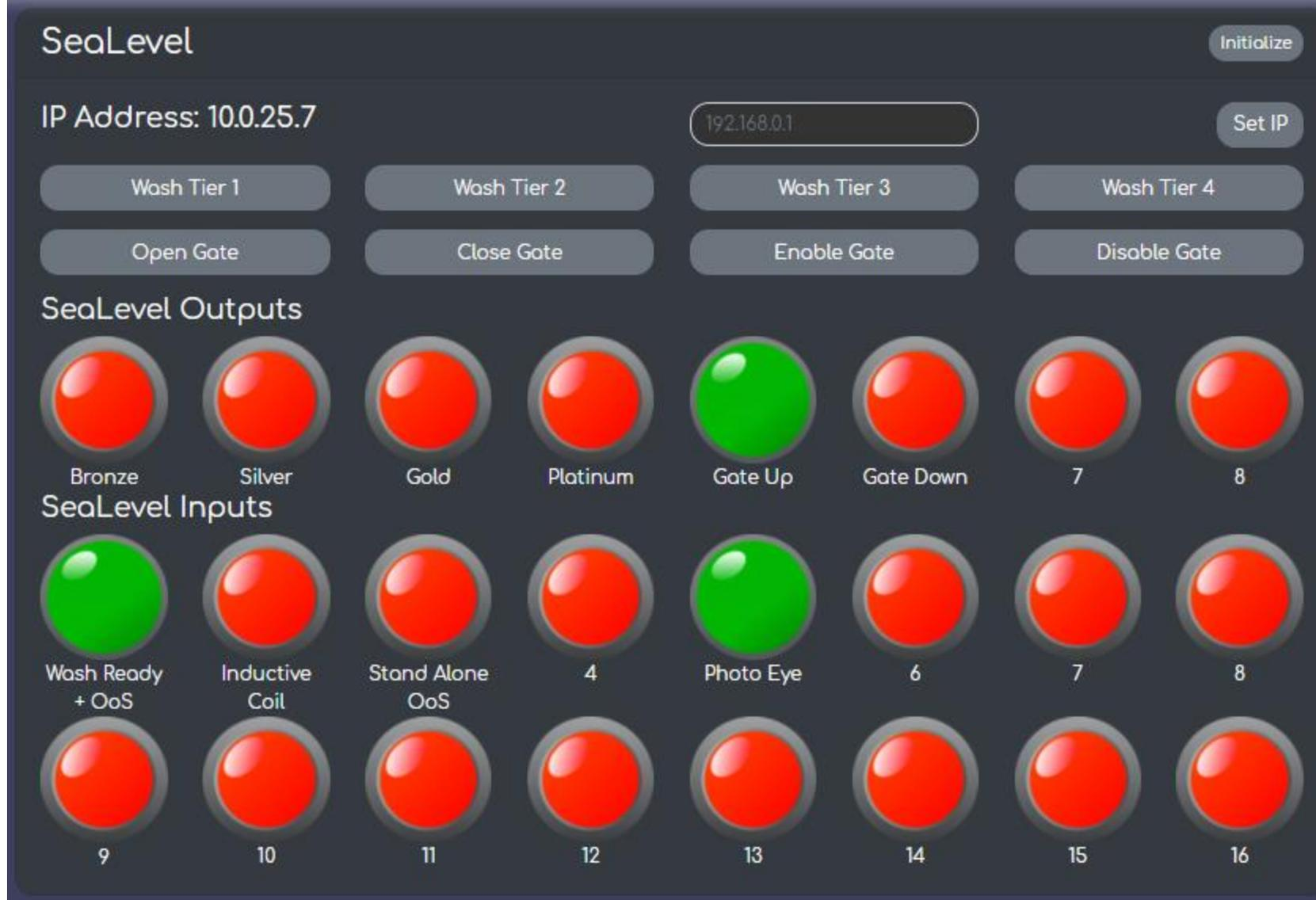
The I/O Interface (a.k.a. SeaLevel) section of the Control Console provides a visual interface between the pay station and the wash equipment. Red and green indicator lights show the current state of each input or output. The gray buttons activate the respective output signal.
