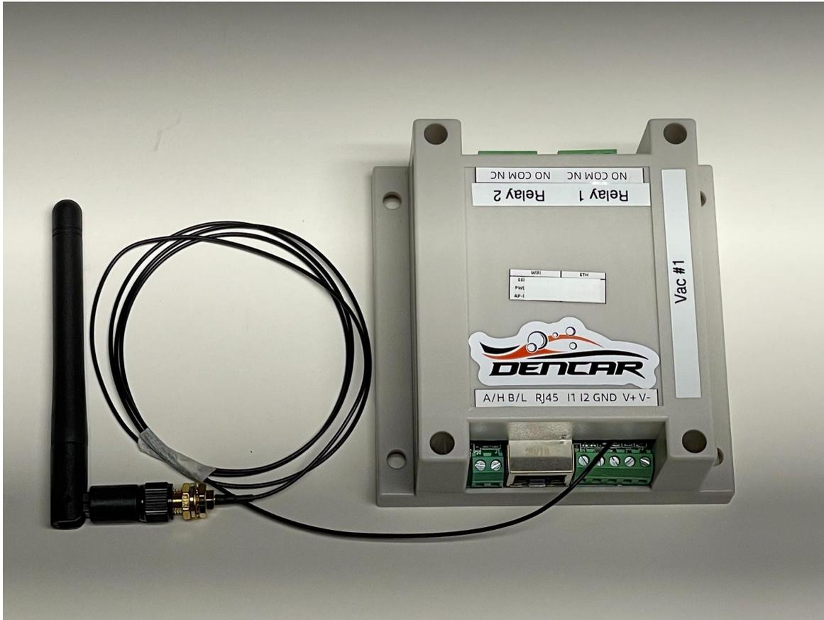
The relay will operate on voltage ranging from 12VDC to 24VDC. Output relay 1 should be connected using the Normally Open (NO) and Common (COM) connections. Wire in parallel to the coin output in the equipment. The relay output contacts are dry contacts and can switch AC or DC up to 10 amps.
