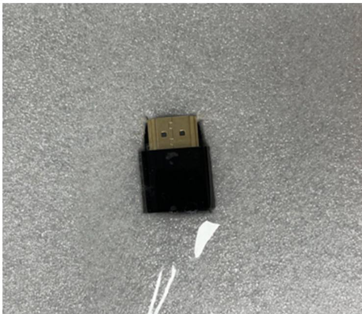
A screen emulator plug is used instead of a full monitor. This plug must be installed so that remote support can be provided.
